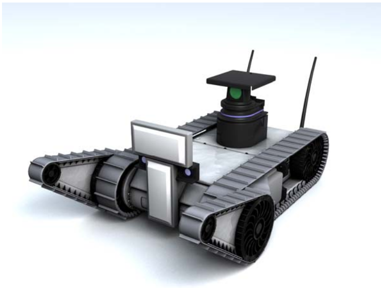
Fig. 1. Daredevil PackBot with polarimetric UWB radar array (concept)
